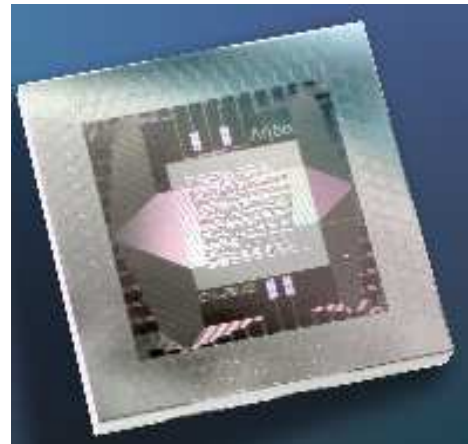
Figure 2. The 28-qubit processor used in the D-Wave / Google Supercomputing 2007 image matching demonstration.
